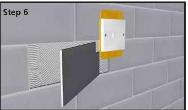
Step 6 Tile with a clean edge to work from. The Safety Shield also ensures sufficient space is left to recess the fitting.
